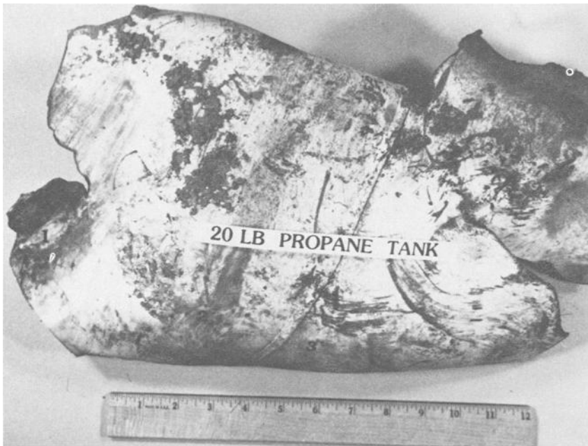
FIG. 9—Photograph of propane tank recovered from near seat of a C4 explosive. Areas labeled 1 to 3 are regions which were examined for presence of RDX and HMX residue with selected ion monitoring.
